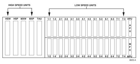
Figure 502-1. Soneplex Broadband Chassis (Front View) Mounting Slot for MPU
